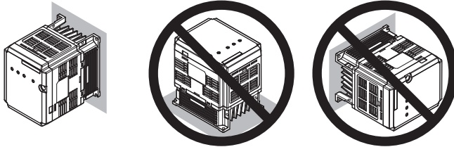
Figure 8 Correct Installation Orientation (Braking Unit)
